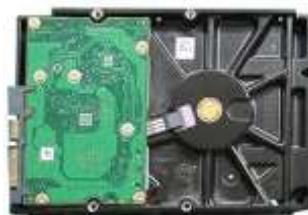
② Fix four screws in the HDD
