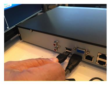
Plug the mouse in to any USB port on the back of the recorder.
