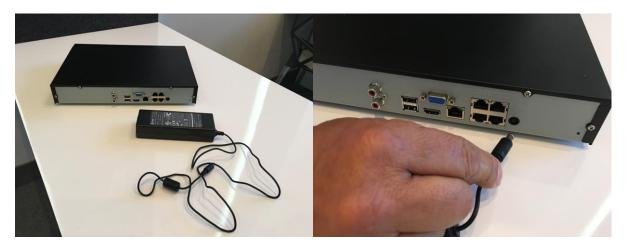
Locate the recorder power supply and plug it in to the rear of the recorder.
