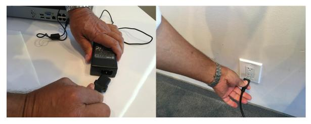
Plug the power wire in to the power supply then plug the power wire in to the wall outlet.
