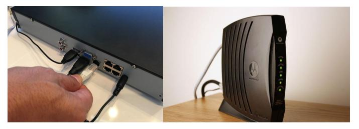
Connect the network cable to the recorder. Connect the other end of the network cable to your Router.
